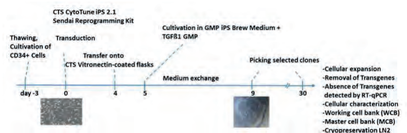
Abb. 3: Timeline of GMP-compliant manufacturing of iPS cells (modified from Dr. A. Haase, LEBAO)
